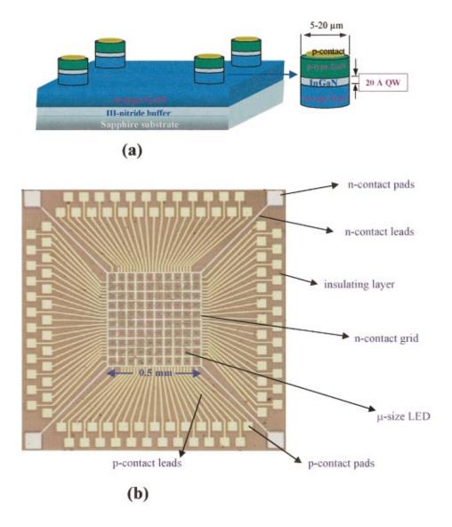
FIG. 1. (Color) (a) Schematic of  $\mu$ -disk LEDs based on p-GaN/InGaN/n-GaN QWs. (b) Optical microscope image (top view) of a microdisplay fabricated from an individually addressed  $\mu$ -disk LED array. The dimension of the microdisplay is  $0.5 \times 0.5 \text{ mm}^2$  (made up of  $10 \times 10$  pixels, 12  $\mu$ m in diameter).
