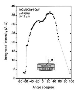
FIG. 4. Angular distribution of light emission from  $\mu$ -disk LEDs measured through the sapphire substrate. The angle is measured with respect to the axis perpendicular to the  $\mu$ -disk surface.
